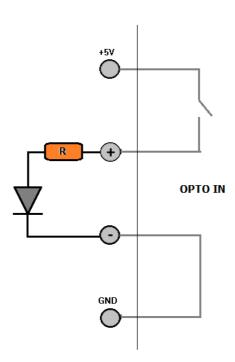
Pin 1-14: Opto 1 IN, command input switching on output 1
